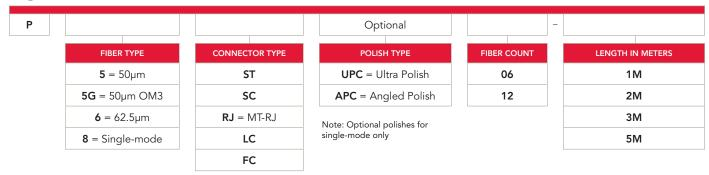
Example: P8SCUPC12-3M = Pigtail assembly, single-mode, SC, ultra polish, 12-fiber, 3 meters in length
